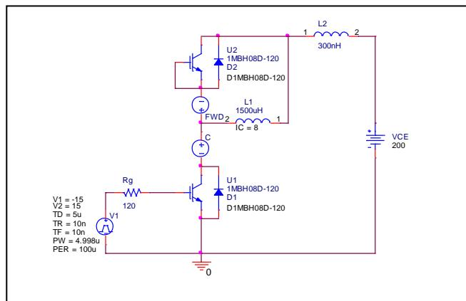
**Test condition:**  $V_{CC}=200$  (V),  $I_C=8$  (A),  $-di/dt= 100$  (A/us)
