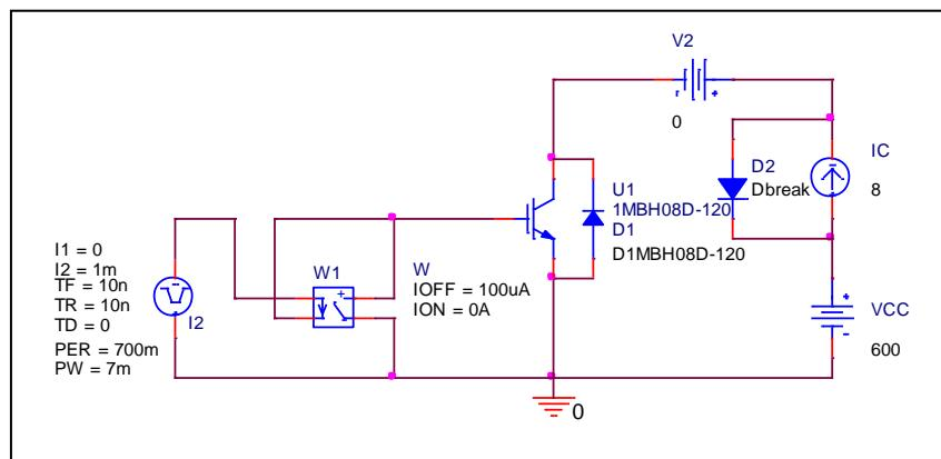
**Test condition: V<sub>CC</sub>= 600 (V), I<sub>C</sub>=8 (A), V<sub>GE</sub>=15 (V)**
