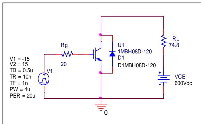
Test condition:  $I_C=8$  (A),  $V_{CC}=600$  (V)
